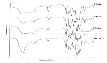
Figure 1. FTIR spectra, for comparison the sulfonyl and benzimidazolyl stretches and their splitting patterns from PANa and its complexes.
