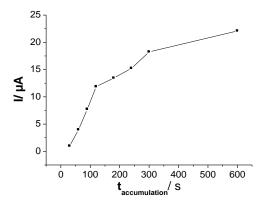
time and sensitivity. In addition, longer accumulation time could also damage the electrode surface that worsens the sensitivity and reproducibility of measurements taken.
