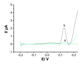
Figure 2. Determination of 4  $\mu$ M Hg (II) by carbon paste (a) and carbon paste modified by extract of takaout (b), E<sub>acc</sub>= -0.9 V, t<sub>acc</sub>= 120 s, equilibrate time= 10 s, frequency = 25 Hz, scan rate= 50 mV/ s, supporting electrolyte 0.1 M acetate buffer, pH = 3.
