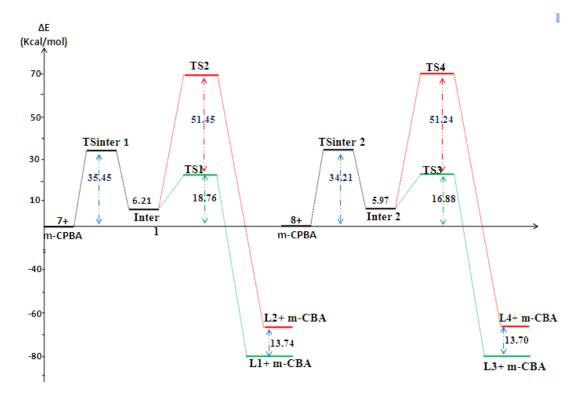
**Figure 2.** Energy profile ( $\Delta E$ , in kcal mol<sup>-1</sup>) of the Baeyer-Villiger reactions of hinikione <u>7</u> and totarolone <u>8</u>
