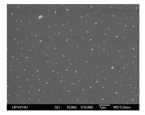
Figure 3. SEM photomicrography of the nanogels.
