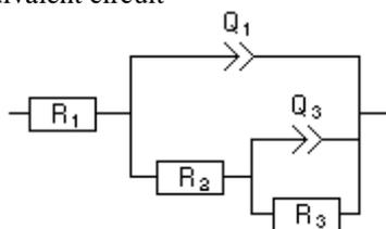
**Figure 3.** The equivalent circuit used to simulate the impedance spectra
