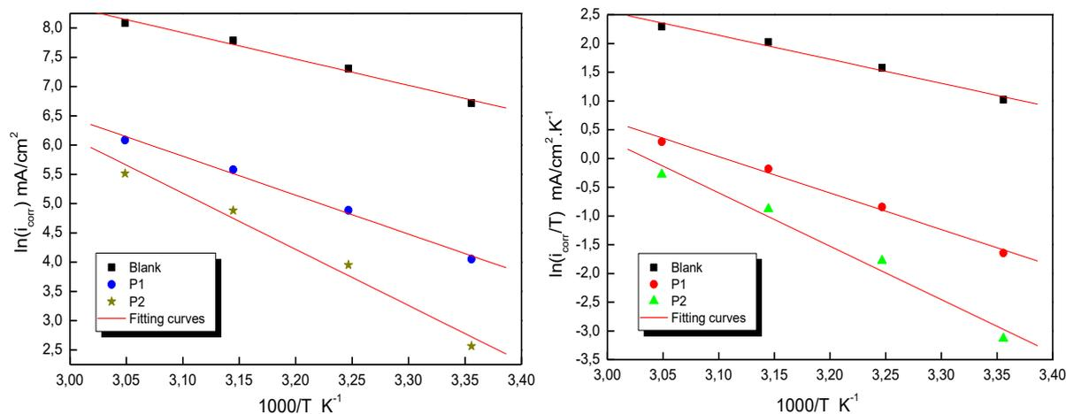
**Figure 5.** Arrhenius lines for stainless steel in H<sub>2</sub>SO<sub>4</sub> 2.0M medium without and with the addition of the compounds P1 and P2 10<sup>-3</sup>M
