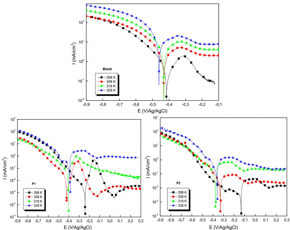
**Figure 6.** Representation of the cathodic and anodic polarization curves for stainless steel in  $H_2SO_4$  2.0M without and with the addition of the inhibitor P1 and P2 at a concentration of  $10^{-3}M$  with different temperatures
