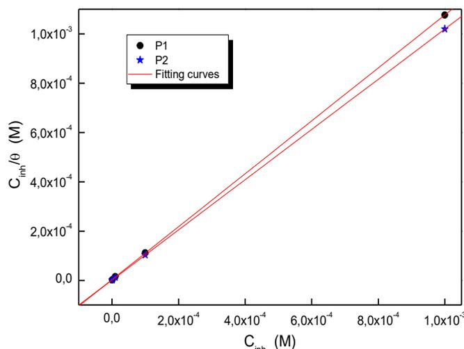
**Fig. 5** The adsorption isotherm of Langmuir for P1 and P2 on the stainless-steel surface at 298 K
