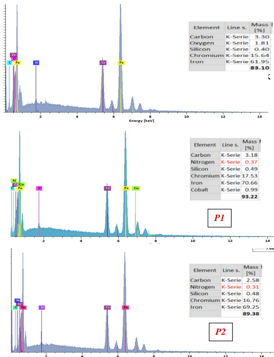
**Fig. 9** EDX spectrum of the steel surface after immersion in a solution containing  $\text{H}_2\text{SO}_4$  2.0M +  $10^{-3}\text{M}$  of the inhibitors P1 and P2 at 298 K
