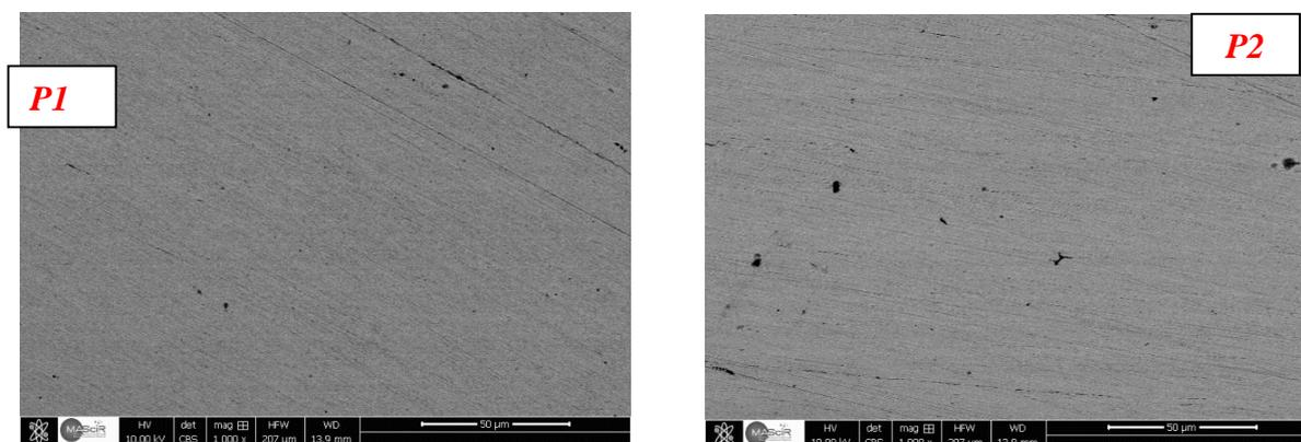
**Figure 7.** SEM images of the steel surface after immersion in the H<sub>2</sub>SO<sub>4</sub> 2.0M medium for 6 hours at 298 K in the presence of 10<sup>-3</sup> P1 and P2
