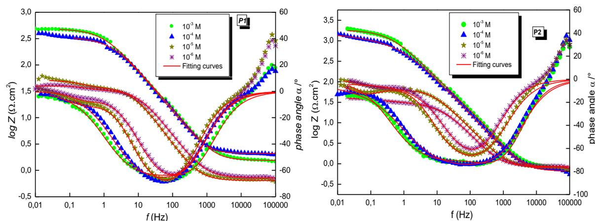
**Figure 4.** Bode spectrum of steel in  $H_2SO_4$  2.0M solution in the absence and the presence of P1 and P2 at different concentrations
