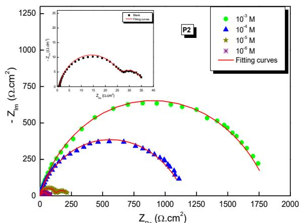
**Figure 2.** Nyquist plots of stainless steel in  $\text{H}_2\text{SO}_4$  2.0M medium without and with different concentrations of P1 and P2
