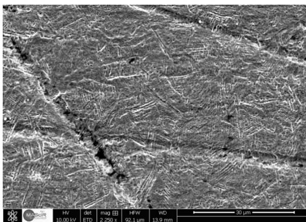
**Figure 6.** SEM images of the steel surface after immersion in the H<sub>2</sub>SO<sub>4</sub> 2.0M medium for 6 hours at 298
