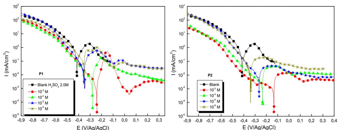
**Figure 1.** Representation of the anodic and cathodic polarization curves for stainless steel in  $\text{H}_2\text{SO}_4$  2.0M medium, in the absence and in the presence of P1 and P2 at different concentrations and 298K
