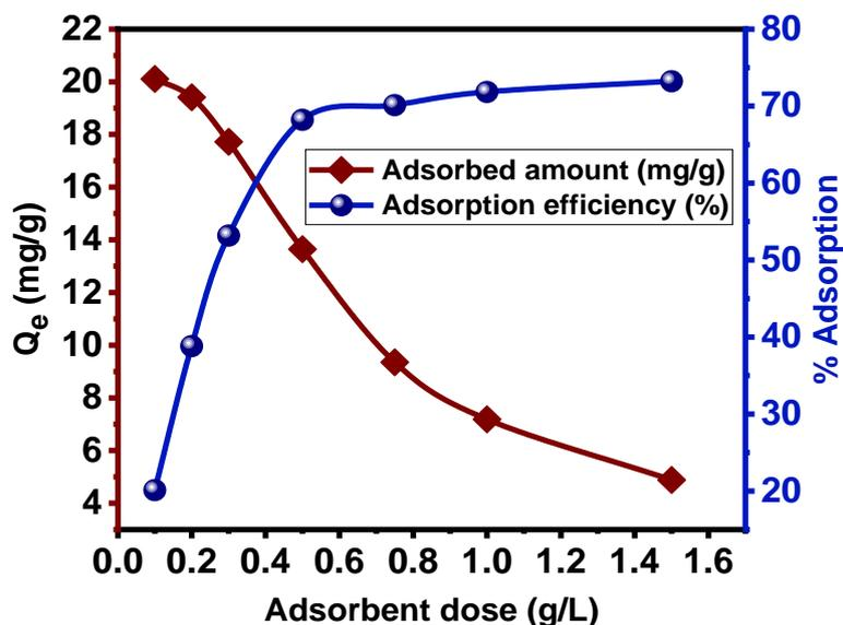
**Figure 3.** Effect of the adsorbent dose on the adsorption of sodium salicylate on the wood sawdust. (Conditions: Contact time = 3 h, C<sub>0</sub> = 10 mg/L, pH = 6.5 and T = 25°C)
