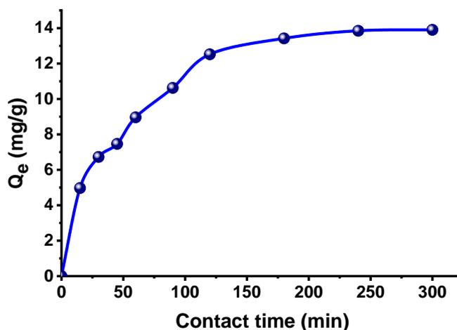
**Figure 1.** Effect of contact time on the adsorption of sodium salicylate onto wood sawdust. (Conditions: R = 0.5 g/L, C<sub>0</sub> = 10 mg/L, pH = 6.5 and T = 25°C)
