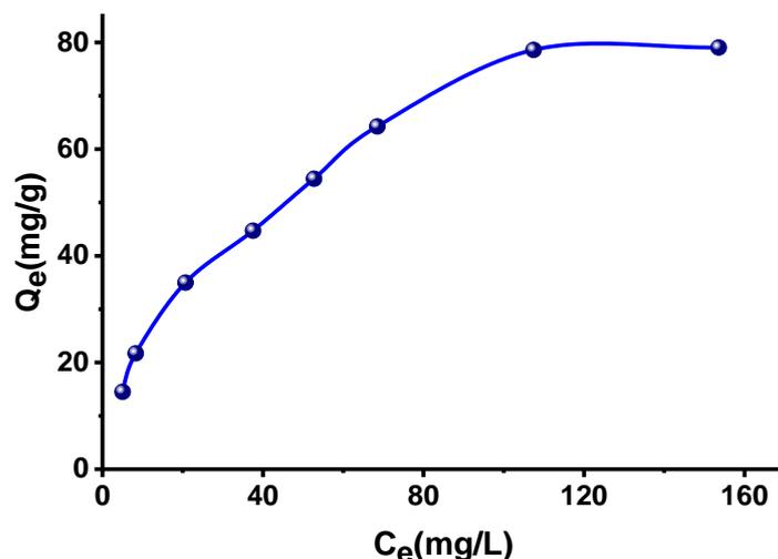
**Figure 5.** Effect of initial concentration on the adsorbed amount of sodium salicylate on the wood sawdust. (time = 3 h,  $R = 0.5$  g/L,  $T = 25$  °C and  $pH = 6.5$ )
