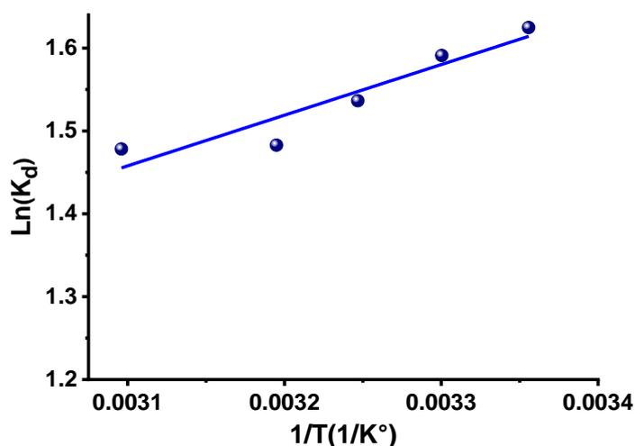
**Figure 7.** Plot of log  $K_d$  vs  $1/T$  for adsorption of sodium salicylate on the wood sawdust**Table 4.** Thermodynamic parameters for the adsorption of sodium salicylate on the wood sawdust.
