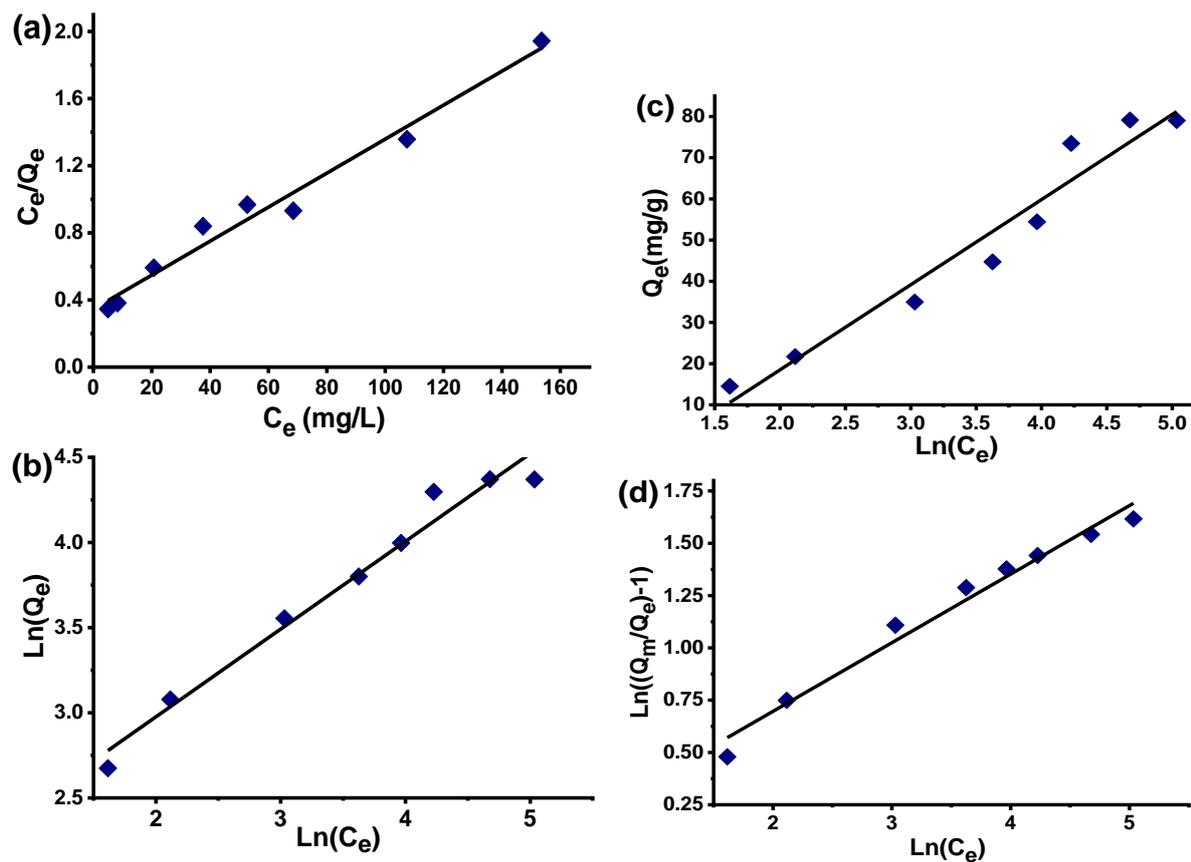
**Figure 6.** Linear plots of (a) Langmuir, (b) Freundlich, (c) Temkin and (d) Generalized isotherms for sodium salicylate adsorption onto wood sawdust
