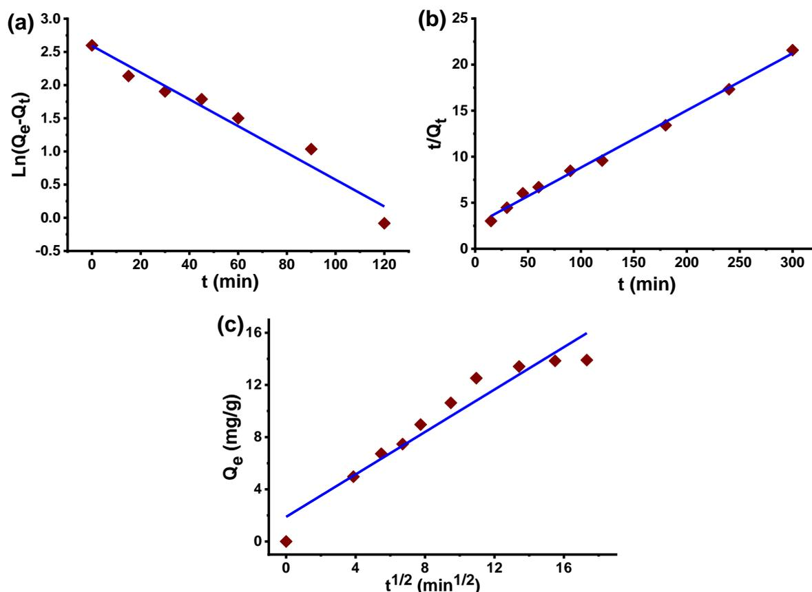
**Figure 2.** Linear plots of (a) pseudo-first-order, (b) pseudo-second-order and (c) intraparticle diffusion models for sodium salicylate adsorption onto wood sawdust
