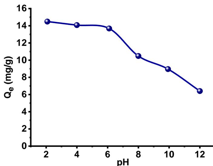
**Figure 4.** Effect of pH on the adsorption of sodium salicylate onto wood sawdust. (Conditions: contact time = 3 h, R = 0.5 g/L, C<sub>0</sub> = 10 mg/L and T = 25°C)
