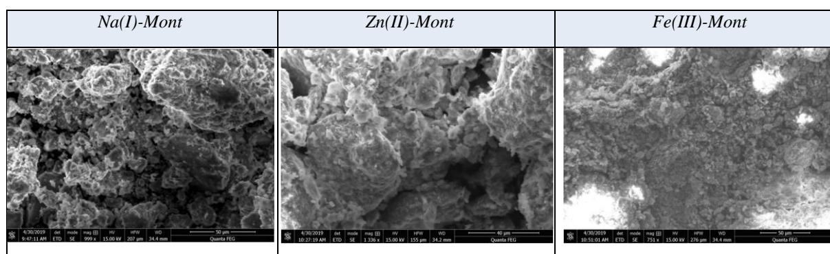
Figure 1. Images of Na(I), Zn(II)- and Fe(III)-Mont recorded by the Scanning Electron Microscope
