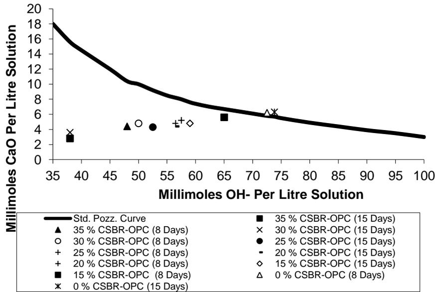
Figure 1: Pozzolanicity Test Diagram for CSBR-OPC
