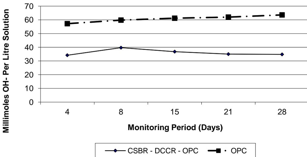
Figure 2:  $\text{OH}^-$  Concentration Change as a Function of Curing Period
