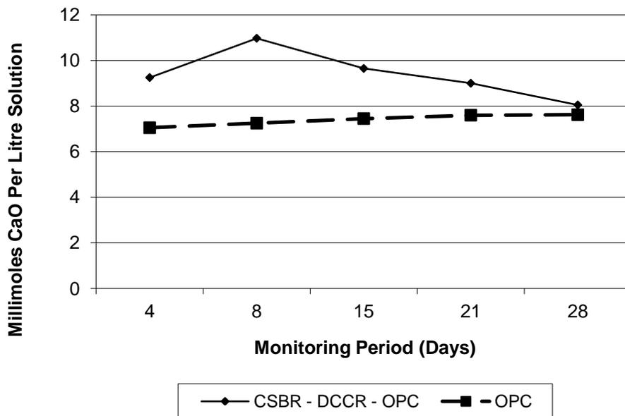
**Figure 3:** CaO Concentration Change as a Function of Curing Period
