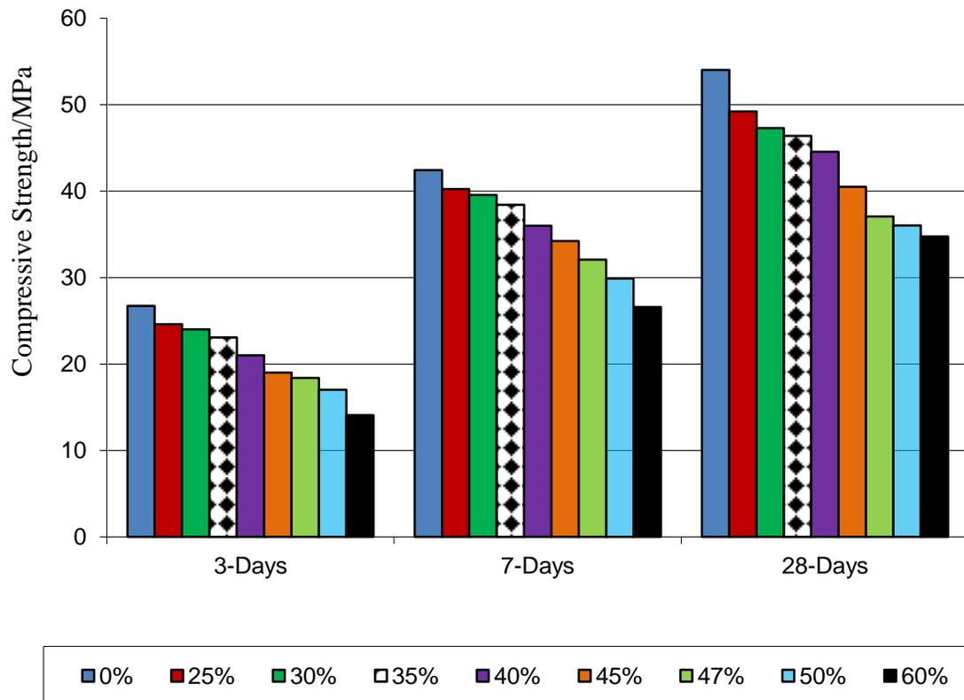
**Figure 4:** Compressive strength Development of CSBR-DCCR-OPC Cement
