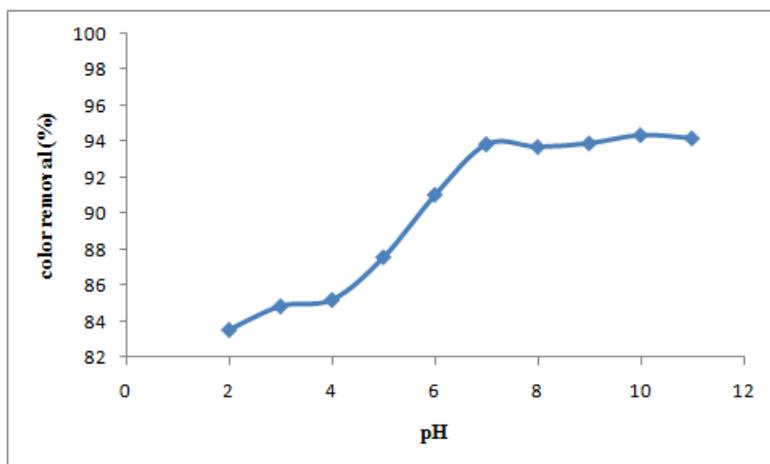
**Figure 5.** Effect of pH on BY 28 adsorption ( $W = 1$  g/L,  $T = 25^{\circ}\text{C}$  and contact time = 3h)
