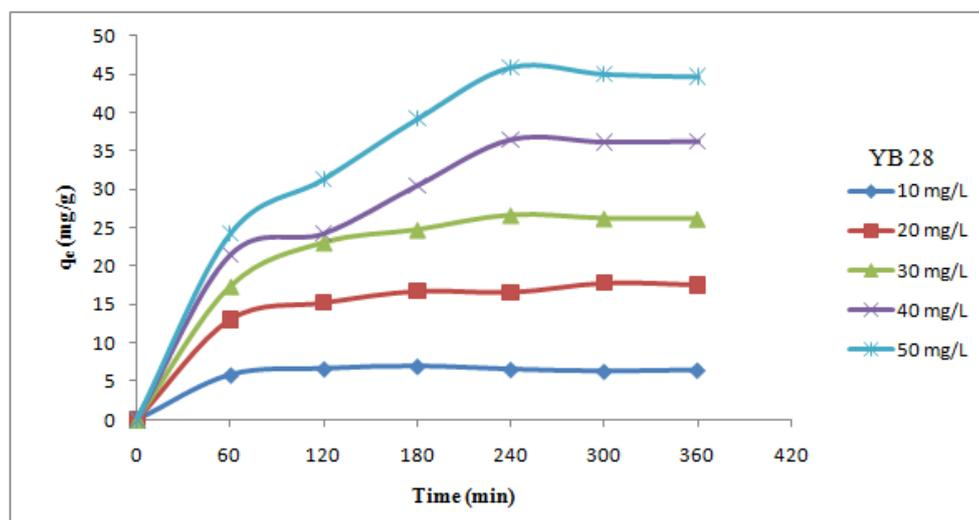
**Figure 4.** Effect of initial dye concentration on BY 28 adsorption ( $W = 1$  g/L,  $T = 25^\circ\text{C}$ , pH initial and Contact time = 6h)
