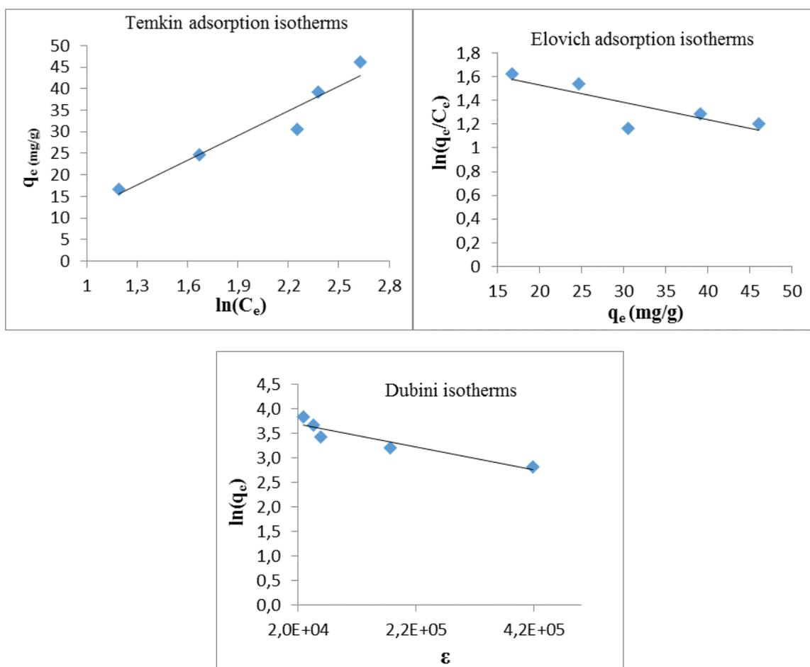
Figure 7. Linear form of isotherm models tested in this study of BY 28 onto CMS.
