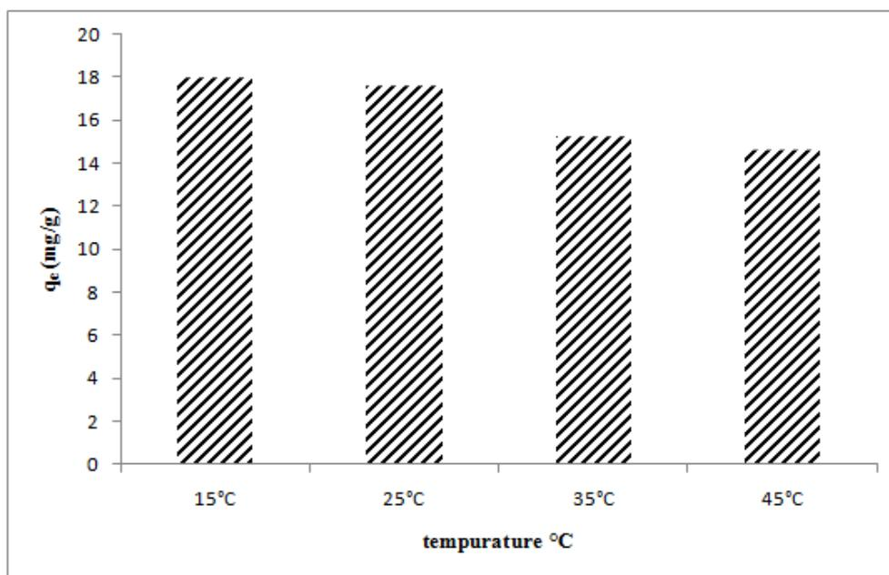
**Figure 6.** Effect of temperature on the adsorption of BY 28 on CMS ( $W = 1$  g/L, pH initial and Contact time = 3h)
