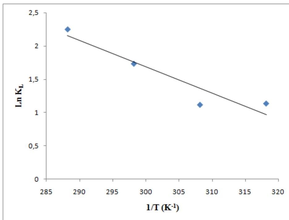
**Figure 8.** Plot of  $\ln K_L$  vs.  $1/T$  for estimation of thermodynamic parameters for the adsorption of BY 28 onto CMS
