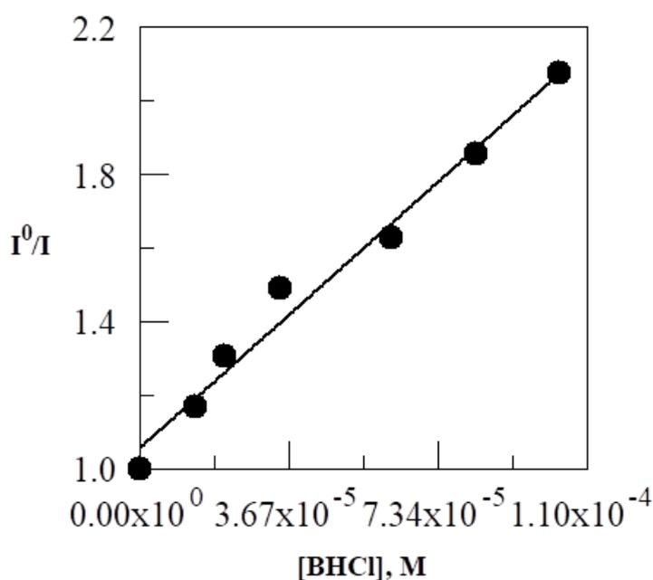
**Figure 6.** Stern-Volmer Plot of the quenching of the Curcumin Fluorescence by BHCl.
